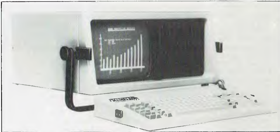
Chameleon (above) claims that it is 'the world's first IBM-PC compatible portable computer that features a dual 8 and 16-bit processor'.
